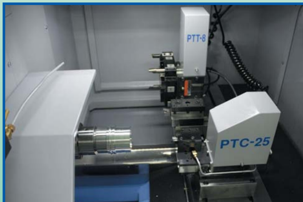
An example of PALLET SYSTEM consisting of PTC-25/PTT-8/ABC tool selection.
